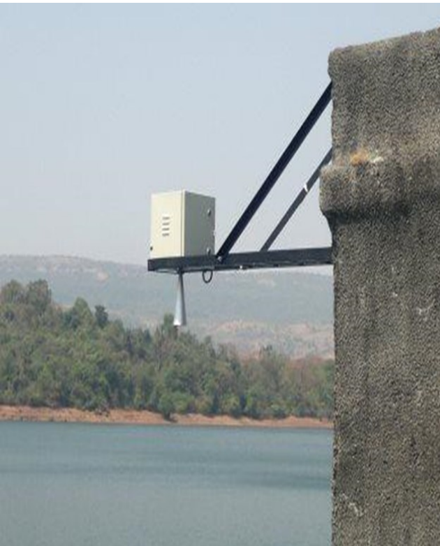
Reservoir Water Level Sensor (RADAR)
